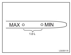
If the oil is at or below the MIN mark, then you'll need to add at least one quart of oil. But you must use the right kind. This section explains what kind of oil to use. For engine oil crankcase capacity, see "Capacities and Specifications" in this section.
